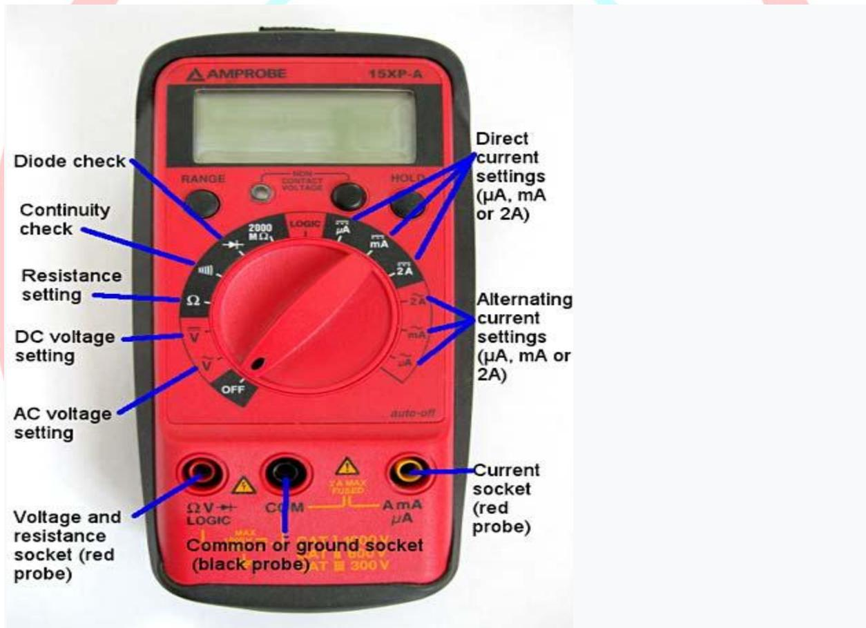
Figure 1.3.1 Digital multi-meters (DMM, DVOM)
