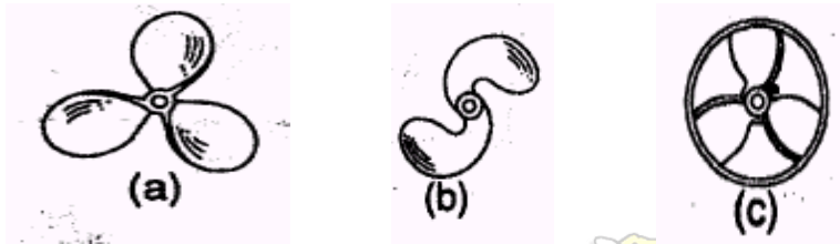
3-blade marine propeller Weedless Guarded stator ring
