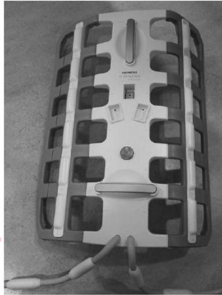
**Figure 5.30** Multi-element body array for 3 Tesla consisting of 24 separate elements. Each element is electrically decoupled from the other individual elements.
