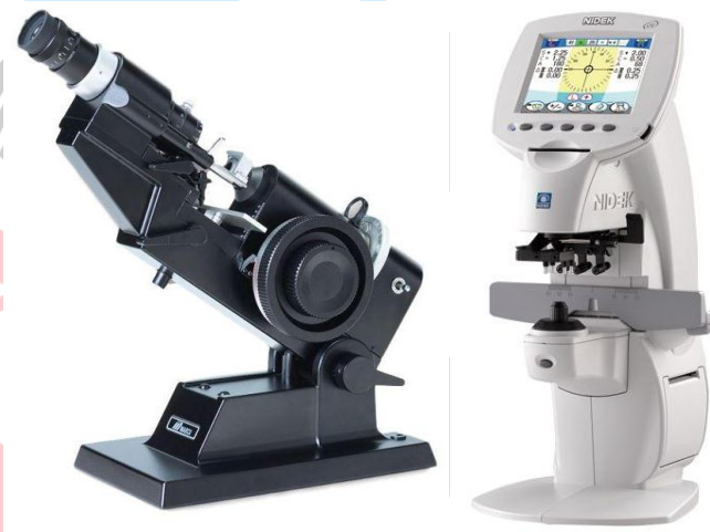
Figure 15 – Manual Lensometer (Left) – Automated Lensometer (right)
