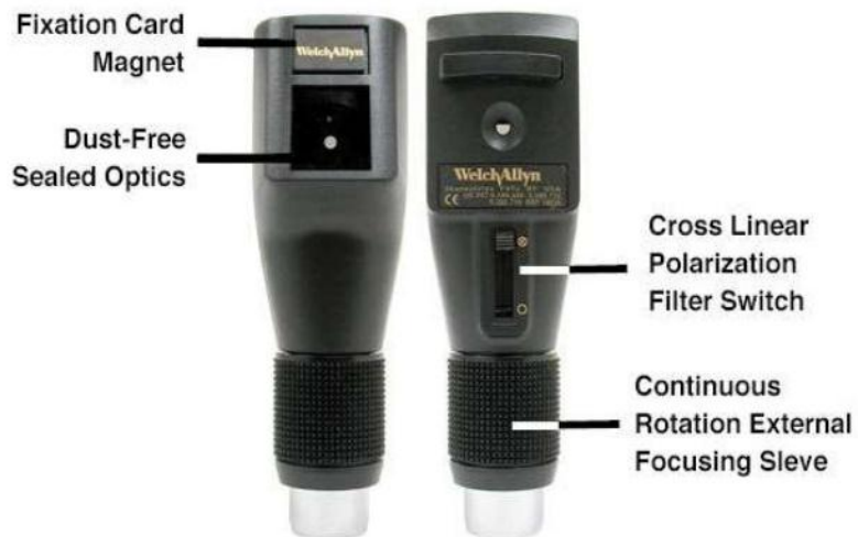
Figure 13- Parts of the streak retinoscope.
